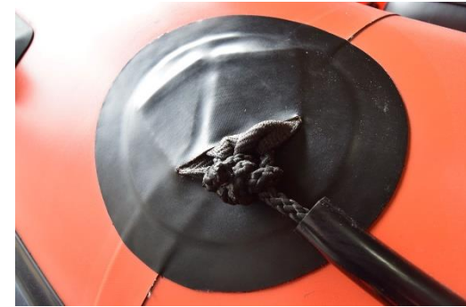
External Life lines mounted on safety line holders
