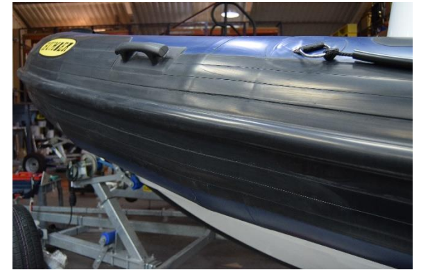
Triple rubbing strake (Flat strake protection above and below standard strake)
