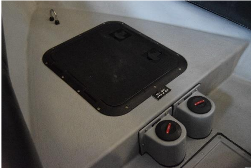
Raised bow stowage locker with two handled access hatch
