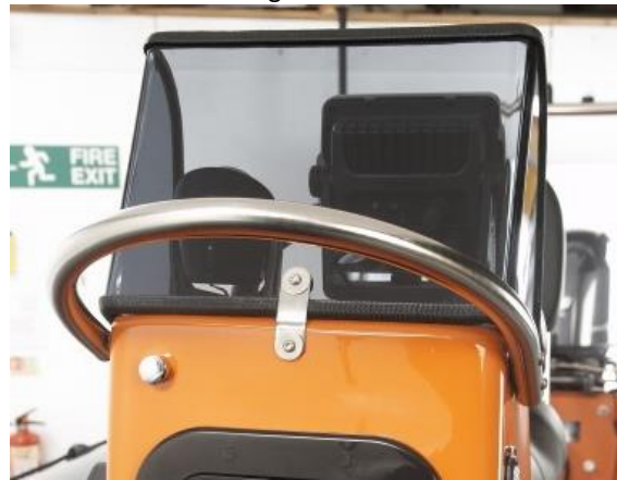
Dual commercial twin helm steering console with deck storage compartment, low screen, over the top & passenger grab rail.
