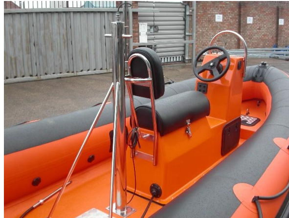
Tow post, tripod with underside bracing Available in stainless steel or black semi-gloss aluminium
