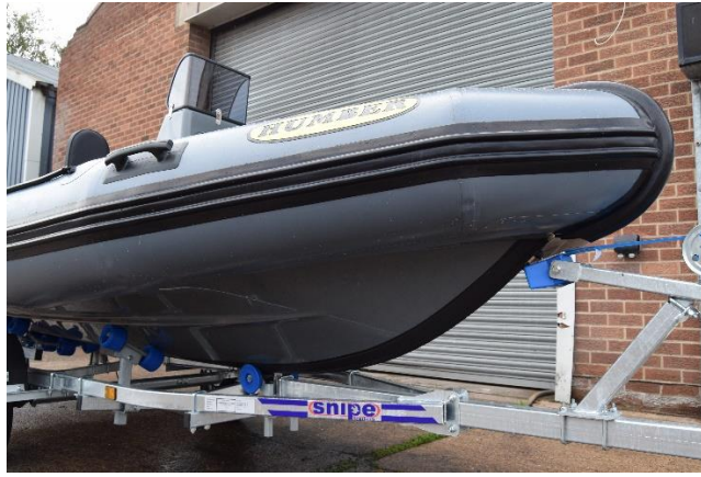
Keelguard bow protection, positioned from underside U bolt 1.5m length
