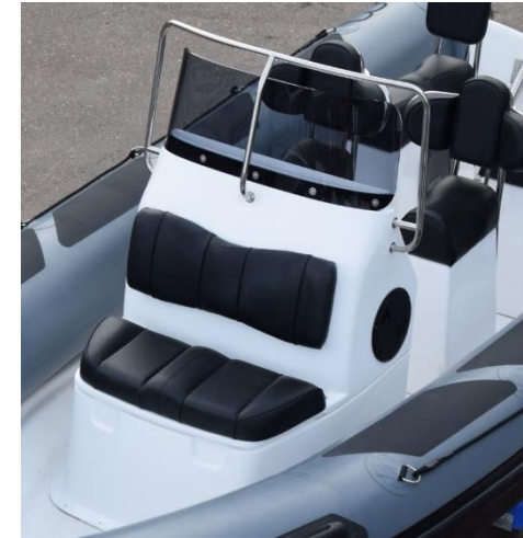
Dual commercial twin helm steering console with deck storage compartment, front twin person seat, low screen, over the top & passenger grab rail.
