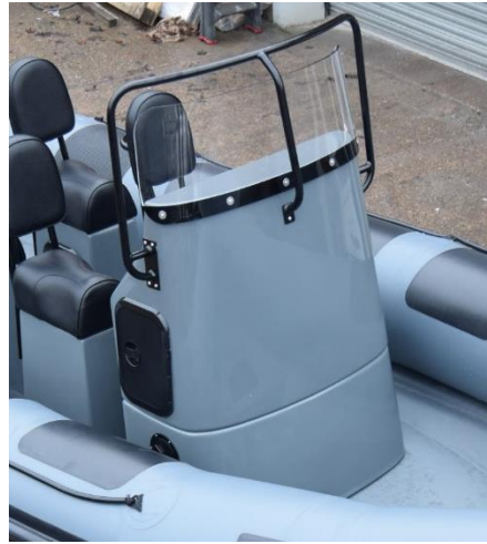
Dual commercial twin helm steering console with deck storage compartment, low screen, over the top & passenger grab rail.
