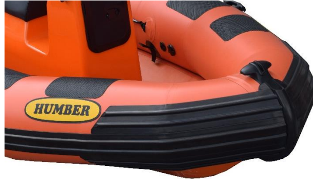
Reinforced bow. Additional strake above and below standard
