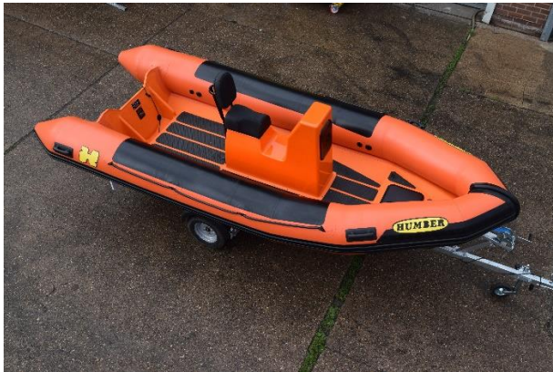
Double skin tube top protection on tube straights, positioned inside front and rear life lines
