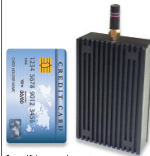
Ranger Mini, a new and compact COFDM H.264 digital video transmitter
